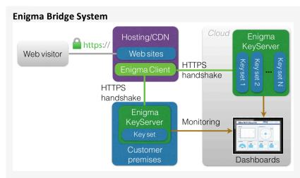
HTTPS Key Service is based around the revolutionary Enigma Bridge KeyServer which has been purpose built to provide high speed access to encryption keys stored on physically partitioned tamperproof processing units (Common Criteria EAL5 / FIPS140-2 Level 3).
